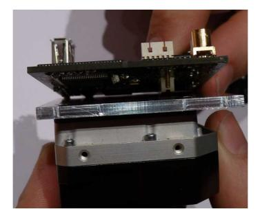
Be careful especially with the both screws near the connector. Tighten the screws not stronger than necessary to keep the board safely connected and in position. Tightening these screws too strong may damage the TAU core or ThermalCapture. After this step the result should look like this:
