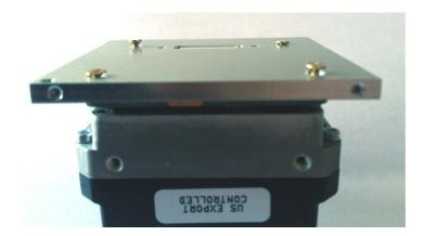
Tighten the screws carefully and make sure that the back plate does not cant. If it cants, loose the screws a little and try again. Do not apply strong forces to screws. After this step your TAU core should look like this:
