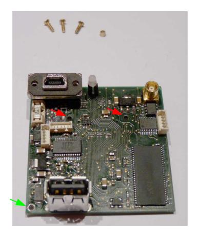
Apply the the insulating discs to two of the screws and stick them through the red marked positions. Stick the screw without insulating disc through the green marked position. Apply the distance sleeve to the screw at the green marked position. The distance sleeve must be added between the board and the ground plate.
