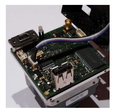
Mount the back cover and attach it with the four M1.6x3mm screws.
