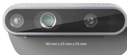
Figura 2: Intel RealSense D435i (<https://www.intelrealsense.com/depth-camera-d435/>)
