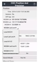
Precision: Users can view horizontal precision, vertical precision and RMS.
