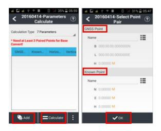
**Note**: Select three corresponding point pairs and add to the interface of parameters calculation.
