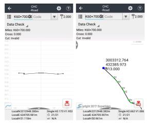
**Free Slope**: When meet slope with same type, users can select free slope to avoid duplication input.
