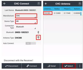
**Auto Connect**: Switch on, then, it will connect previous device when users open the software.
