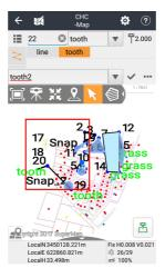
**Survey Boundary**: Click to view survey boundary interface, users can select several points to build boundary. Settings of survey boundary are for planning out one job area.
