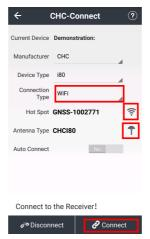
**Demonstration**: Enter Demonstration mode, and then users can use or test all the functions of this software. Meanwhile, the function can simulate position by inputting coordinate.
