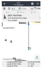
Arrow: Give direction to target point in real time.
