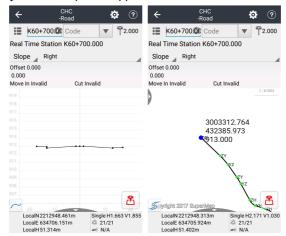
**Data Check**: Use receiver to check any position on roads whether it remains deviation.
