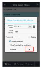
Then the green LED will flash and the states will come from **Single** to **Fix**, which means the rover is getting the correct data from base.
