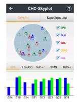
**Satellites List**: Users can view the current number of each satellite which has been searched, constellation, L1 \ L2 \ L5 SNR, elevation angle, azimuth, and locked status information.
