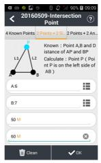
**Points + 2 Angles**: Calculate intersection P with known points A and B and the inner angle of PAB. Click **OK** to calculate. Input a name, and click **OK** to save.
