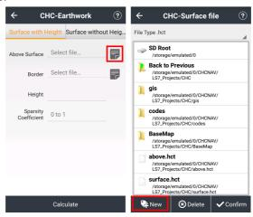
Users can choose surface file or create a new surface file by selecting points. Click **New** to create a new surface file, users can add a new point or select point in **Points**, then click **OK** and save new surface file. The storage path of new surface file is: CHCNAV/LS7 Projects/CHC/.
