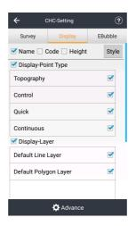
Name/Code/Height: Select to display on Map interface, users can select one item or multi-item. For example, if selecting Name and Code, users will see point name and code on Map interface after measurement.
