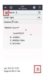
**Setting**: Click to set parameters (See details in 4.1.2). After all parameters set, tap **Measure** (The red icon in down-right corner of interface) to start surveying work.
