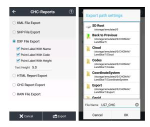
**Note**: After exporting DXF file, you can see shape folder (including .dxf and .shx files) in the same root catalogue of DXF file, please copy both DXF file and shape folder to your computer (must be in the same root catalogue), then correct codes of DXF file will display in your computer.
