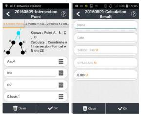
**Points + 2 Sides**: Select points A and B from point management. Enter the length of line AP and line B. Click **OK** to calculate. Input a name, and click **OK** to save.
