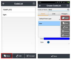
Click **Layer** and enter the interface of **Layer Manager**. Click **New** to enter the interface of **Create Layer**, input layer name and type, select color, size and style, add description. Click **OK** to complete.
