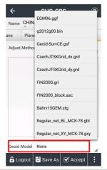
**Note**: Users should put geoid files in following path: CHCNAV/LandStar 7/Geoid. Then restart LandStar 7 to apply geoid files. Users can download regional geoid files from following URL:
