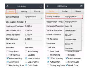
**Survey Method**: Support topographic point, control point, quick point, continuous point, offset point, compensate point and corner point.
