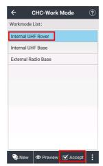
Then the green LED will flash and the states will come from **Single** to **Fix**, which means the rover is getting the correction data from base.
