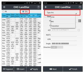
Line: Input azimuth and length.
