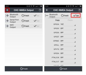
Please ensure Baud rate is 9600 when GPGGA Serial output set is 1HZ based on connecting CHC Receivers.
