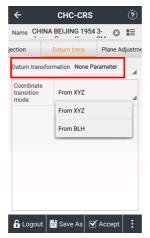
**7 parameters**: Requires at least three known points, and the points can be under the national coordinate system or the coordinate system that existing small rotation from the WGS84 coordinate system. Preferably three or more
