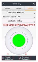
① **EBubble Calibration**: Click to get the offset info of the receiver. When the offset angle is less than the limit value, users can click OK, and then start EBubble calibration.
