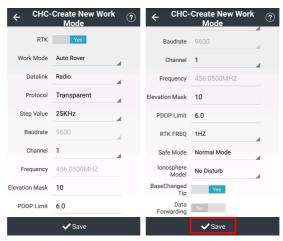
**Data Forwarding**: Forward data through Bluetooth, Serial Port, WIFI, and Radio Station.
