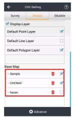
**Advance**: Configure what else to display by advance selection. Users can filtrate through single point or multiple points or height.
