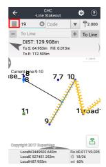
Click list to enter the line library management, users can input the point directly, or users can add customized points from the point management, including three linear types: lines, circles, arcs.
