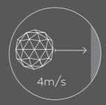
Elios' protective frame is made up of carbon fiber covered with a soft coating. It can sustain collisions, evenly, all around the drone at a speed reaching up to 4 m/s.
