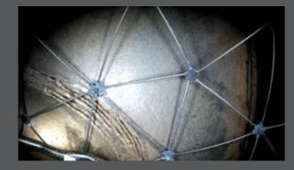
When flying in contact with a surface, Elios can gather close-up images with a sub-millimeter resolution of 0.2 mm/px.
